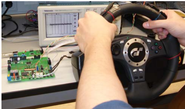
Fig. 3. Implemented system running. In the steering wheel there are two ECG electrodes and the presure sensors connected to the hardware.
